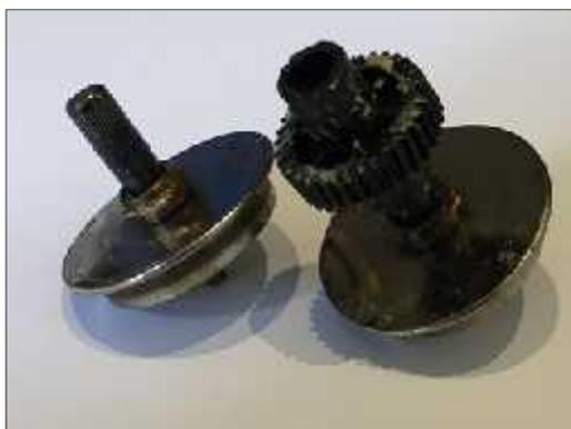
With the judicious use of a hair dryer or hot air gun, a scrap USA Trains axle can be separated into two wheels and the brass bearings pulled off the axle.
